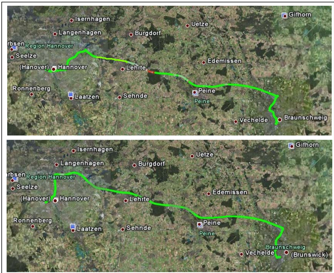
Figure 4: Reception while driving 120kmph, between Hannover and Braunschweig. Top picture shows reception quality when using single antenna receiver. Bottom picture shows reception quality when using two antennas receiver. Similar impact was obtained in trials in China, with CM-MB.
