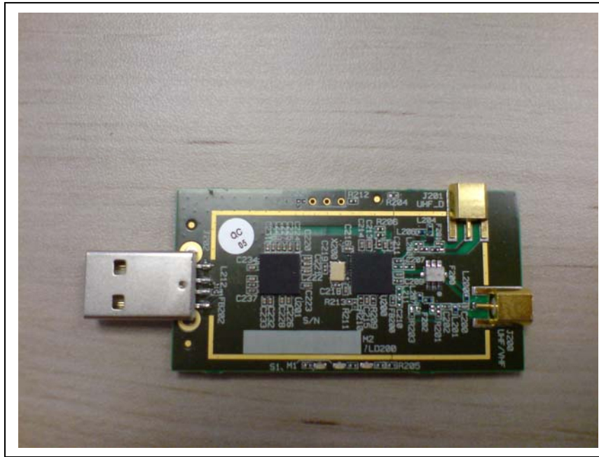
Figure 6: Diversity solution based on Siano's SMS1230 receiver with the SMS1205 diversity companion
